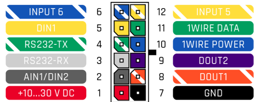
Figure 2 FMU125 2x6 socket pinout
